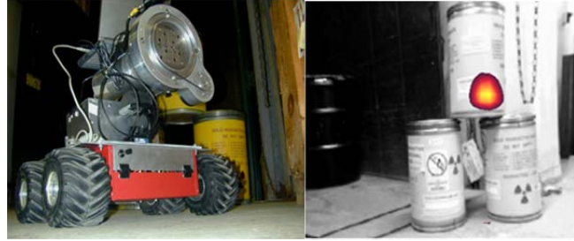
Figure 1 (Left) Remote RadCam system tested at University of Michigan nuclear reactor. (Right) The RadCam image recorded at the University of Michigan nuclear reactor service room of the filtrations system and waste storage drums. The image shows the location of radioactive material in the drums.
