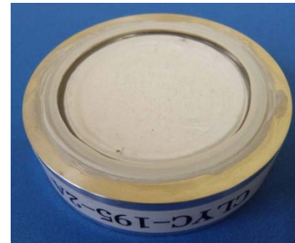
Figure 3 Picture of the 2-inch diameter, 5mm thick CLYC crystal packaged in an airtight package.
