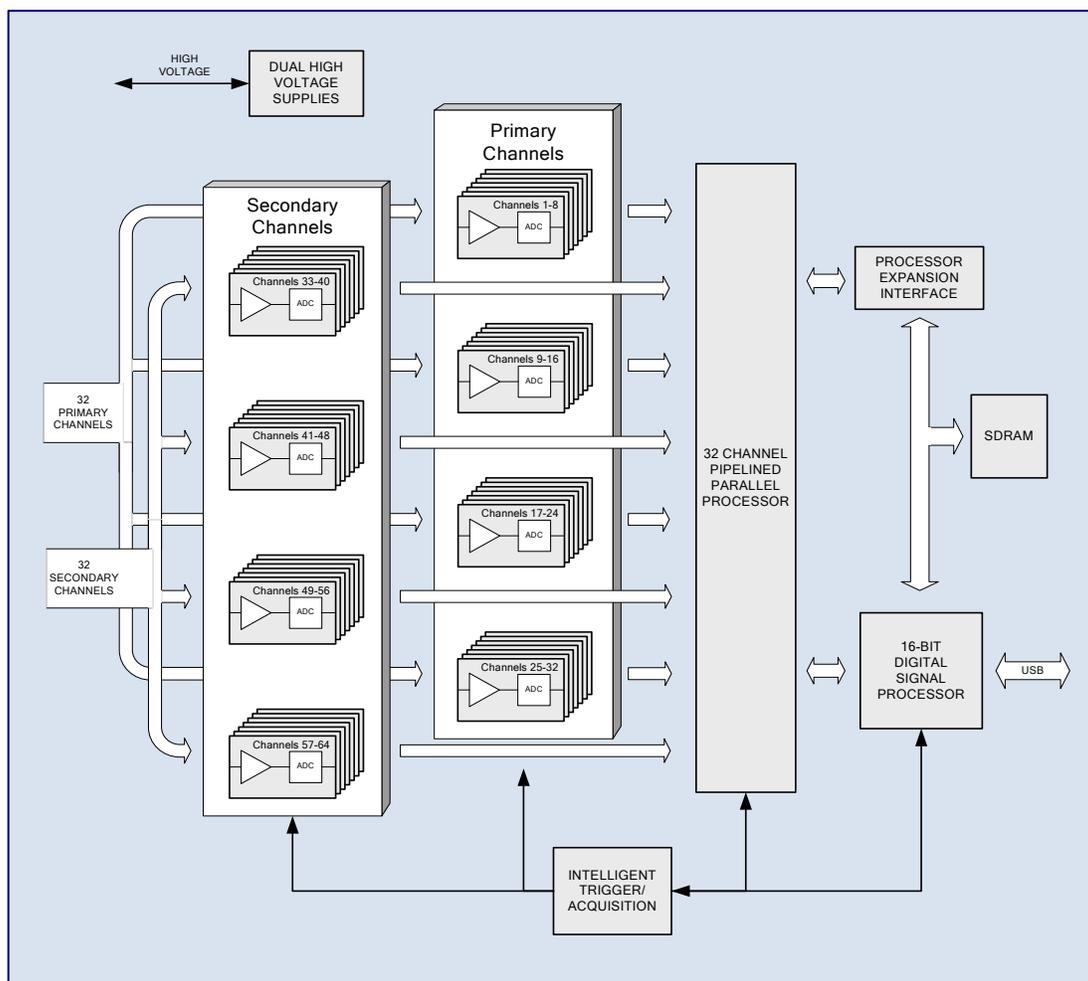
PhotoniQ Functional Block Diagram
