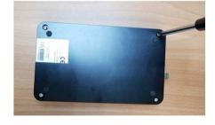
Unscrew these 4 screws on LS-DH-2. (Place SMA905 to the right direction is recommended)
