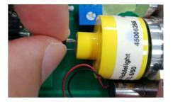
Plug the power cord of halogen lamp. The power cord is no positive/negative difference.
