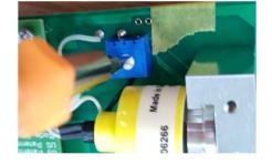
Use Flathead screwdriver turn clockwise and counterclockwise to enhance or reduce the intensity of halogen light.
