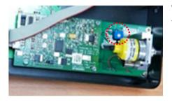
The left picture shows the position of the blue variable resistor.
