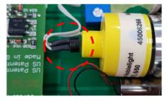
Remove the power cord of halogen lamp.
