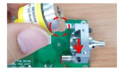
Install the new lamp and please note there is an error-proofing design as shown in the left picture.
