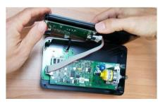
Disassemble the bottom Cover. (It is no need to disassemble the cable)
