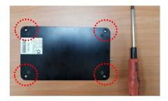
There are 4 screws located at the bottom of the LS-DH-2, as shown in the left picture.
