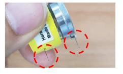
There are two power supply pins of deuterium lamp located at the bottom of the lamp.
