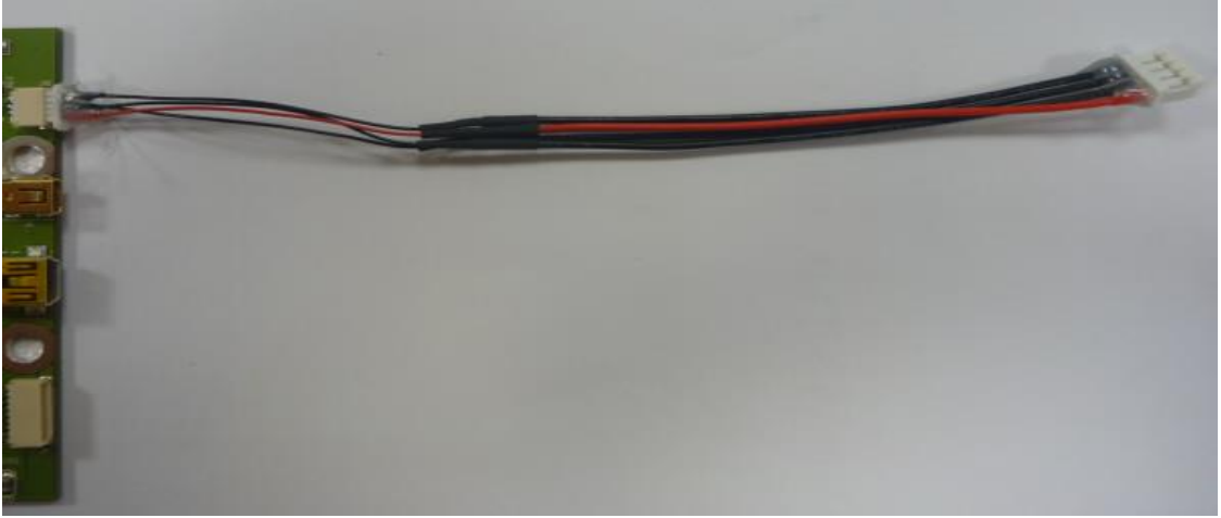
Fig. 6: UART Port Extension Cable Picture
