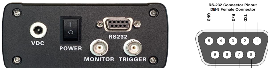
Figure 7 – Rear Panel with DB-9 Pinout (RS-232)
