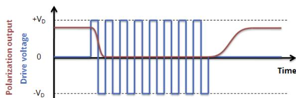
\* The PolarSpeed®-M(L) model shows inverted optical response, i.e. non-altering without voltage applied.
