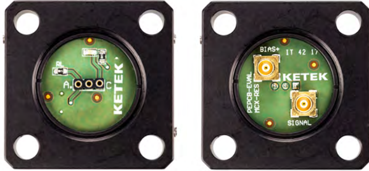
Fig. 2 PEPCB-EVAL-MCX-RES-P Connection Scheme
