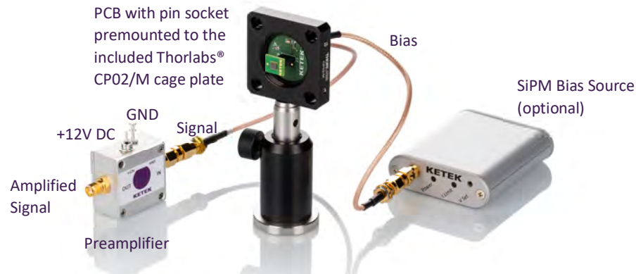
Fig. 1 PEVAL-KIT-MCX Connection Scheme
