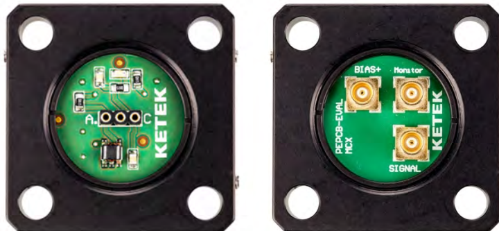
Fig. 3 PEPCB-EVAL-MCX-P Connection Scheme
