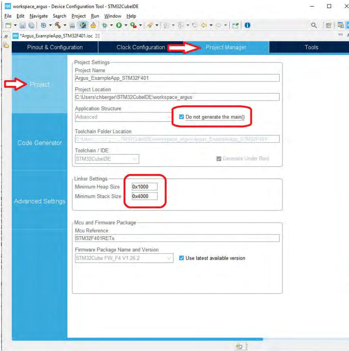
Figure 30: Forcing Separate Initialization Files
