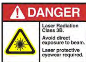
Figure 7: Laser Safety Warning Sign for Unrecommended/Nondefault Operation
