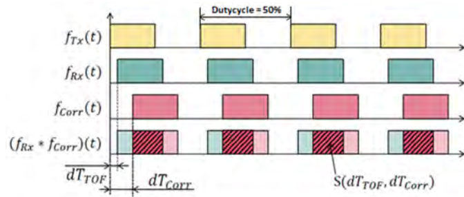
Figure 2: iToF Correlation Schematic
